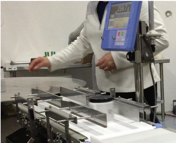
Production line checkweighing at Atlas Putty
